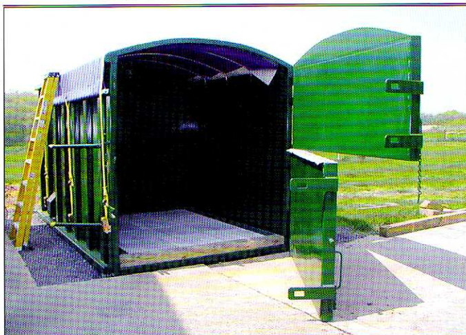
Figure 1: Aerated floor vessel, showing the aeration chamber. Instrument room is in the rear of the vessel.
